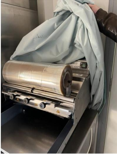
A photograph of a stainless steel tray packaging machine. A roll of clear plastic film is being fed into the machine, which is partially covered by a light blue cloth. The machine has several rollers and a control panel. | 200 |
