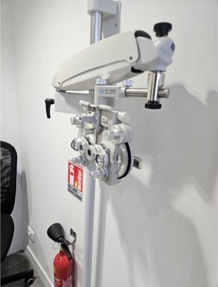
A photograph of a white NIDEK RF 600 head of a refractometer. It is a complex mechanical device with multiple lenses and adjustment knobs, mounted on a vertical metal stand. The device is positioned in a clinical setting with a white wall and a red fire extinguisher visible in the background. <p data-bbox="1445 1151 1493 1180">600</p> |              |
