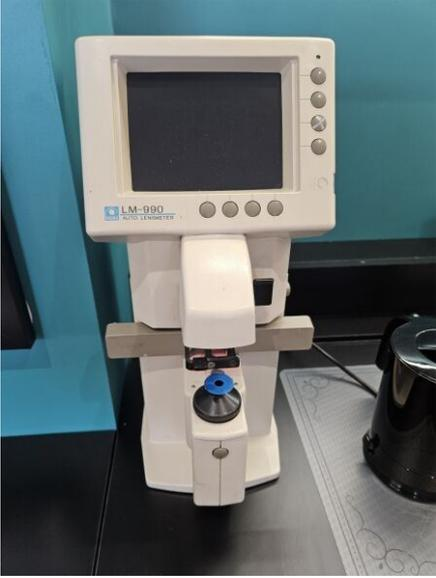
A photograph of a white NIDEK LM 990 frontofocomètre. It features a large monitor at the top with a dark screen and several control buttons to its right. Below the monitor is a white frame with a blue lens and a patient's chin rest. The device is placed on a dark surface against a light blue wall. <p data-bbox="1445 488 1493 517">300</p>     |              |
