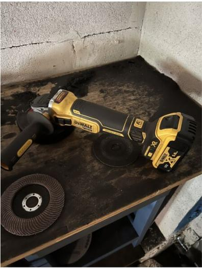
A yellow and black Dewalt battery-powered angle grinder with a grinding disc attached. It is lying on a dark wooden workbench. Another grinding disc is visible next to it. <p>60</p>                                        |
