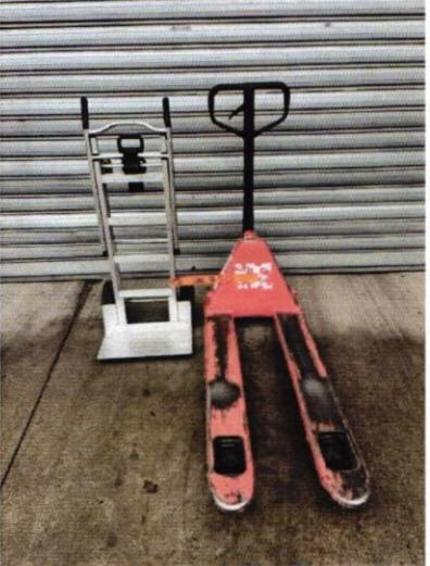
A photograph showing two pieces of manual handling equipment. On the left is a white hand truck (diable) with a single vertical mast. To its right is a red pallet truck (transpalette) with a horizontal mast and a large triangular base plate. They are positioned on a concrete floor in front of a light-colored corrugated metal garage door. |
